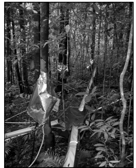
Above: Typical cloud forest environment Left/right: Equipment for measuring stemflow and throughfall being set up in the forest
