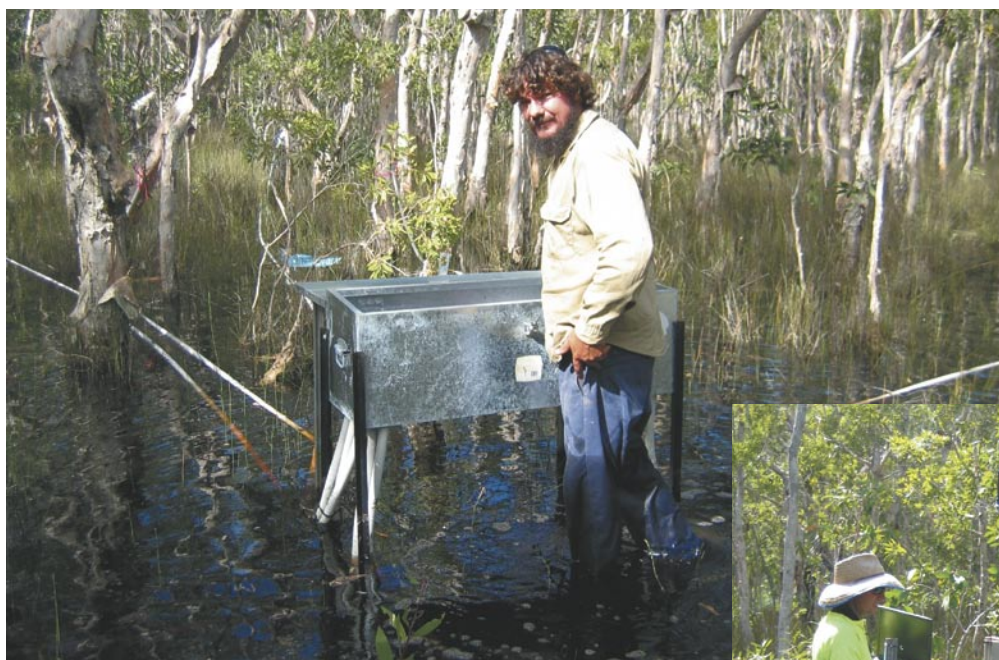
Left: Mark Disher checks heat pulse instrumentation for measuring water use of inundated Melaleuca swamp at Cowley Beach.
