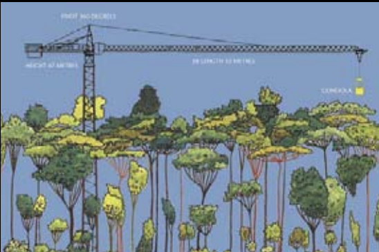
A conceptual diagram, showing the set up of the crane in relation to the forest canopy.
