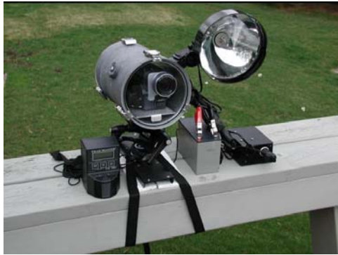
Figure 16. Trailmaster TM700v Passive Infrared Video Trail Monitor with remote sensor (Photo: Professor Kerry Foresman).
