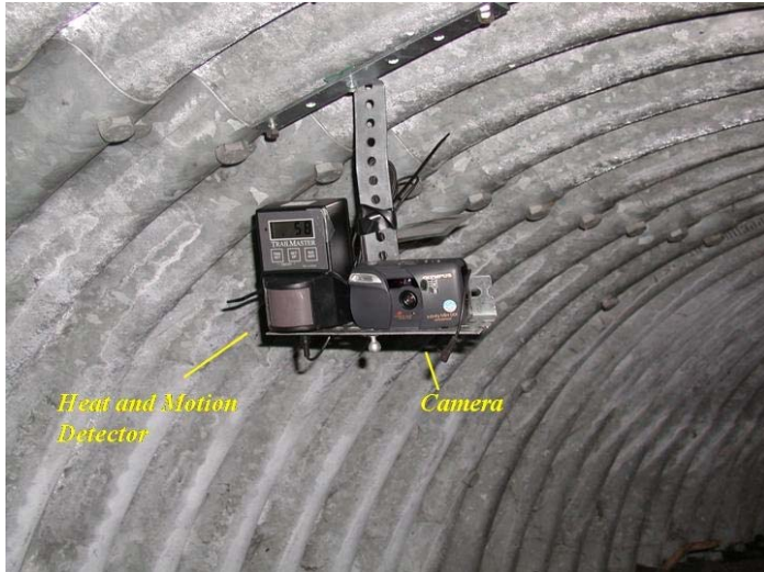
Figure 13. Trailmaster camera with passive infrared sensor mounted on roof of culvert (Photo: Professor Kerry Foresman)
